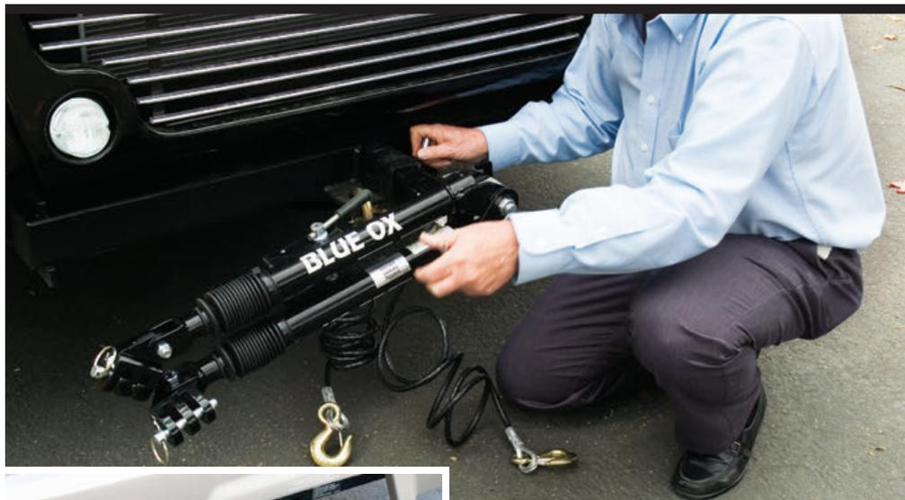
Above: Once the tow bar is pinned in the hitch receiver, make sure electric connections and safety cables are secure. Left: While driving the dinghy, this type of tow bar remains on the coach, out of harm's way.
