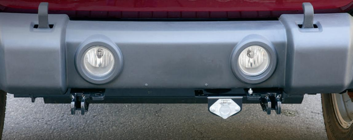
▲ Modern baseplates are secured to the frame of the dinghy. While some installations are more complicated, the end result usually is a clean appearance.
