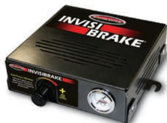
ler is installed beneath the front seat of the towed vehicle. An air cylinder is installed close to the controller; a bracket and cable pulley are installed on the brake pedal arm. The entire system is designed to stay in the vehicle.
