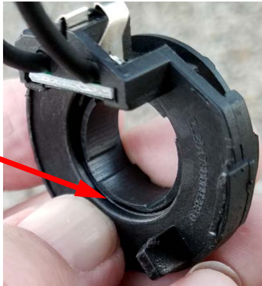
Figure 10: Photograph to Illustrate the Gap Space Between the LED Socket on Adapter
